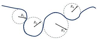
An arbitrary trajectory is divided into different arcs of a circle  $(R_i)$
