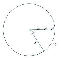
$l_1 < l_2 < l_3$ Rotation angle  $\varphi$  radians  $\varphi_1 = \varphi_2 = \varphi_3$  $\varphi = \frac{l_0}{R}; \quad l_0 = \varphi R$  (1)
