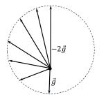
**NO:** At the moment of time when the vector of total acceleration is horizontal, its projection on the vertical axis is equal to O
